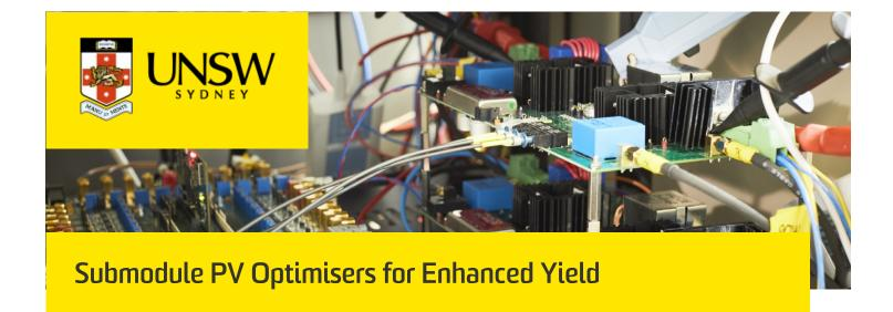
Developing power electronic-based optimiser circuits that maximise the energy output, in real time, from photovoltaic panels that have become shaded, hot or are deteriorating. Doing so attacks the costs and benefits of PV systems from two significant directions, improves the yield and enhances the return on investment.
