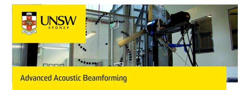
Advanced methodologies for the localisation and characterisation of sound that can be used in challenging environments, such as wind tunnels, hydroacoustic testing tanks and factories, to improve the design of aircraft, submarines and wind turbines.
