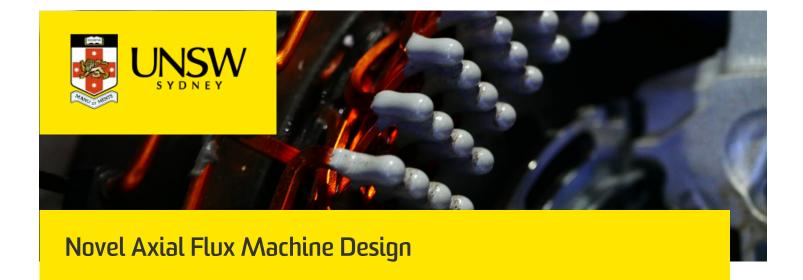
The development and assessment of ground-breaking and innovative axial machines. Axial flux machines have a form factor that suits inhub motors for electric vehicles. They have been used for many years as the motor of choice for the world record-breaking Sunswift team, and are a popular choice of electrical generators for small- and large-scale wind turbines.
